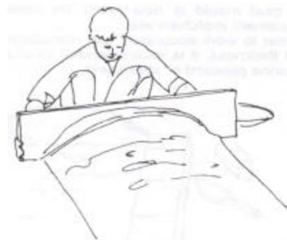
A template is used to get the exact shape of the mould
