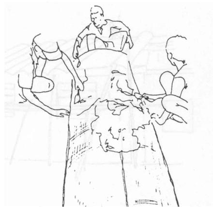
Applying the second layer of mortar
