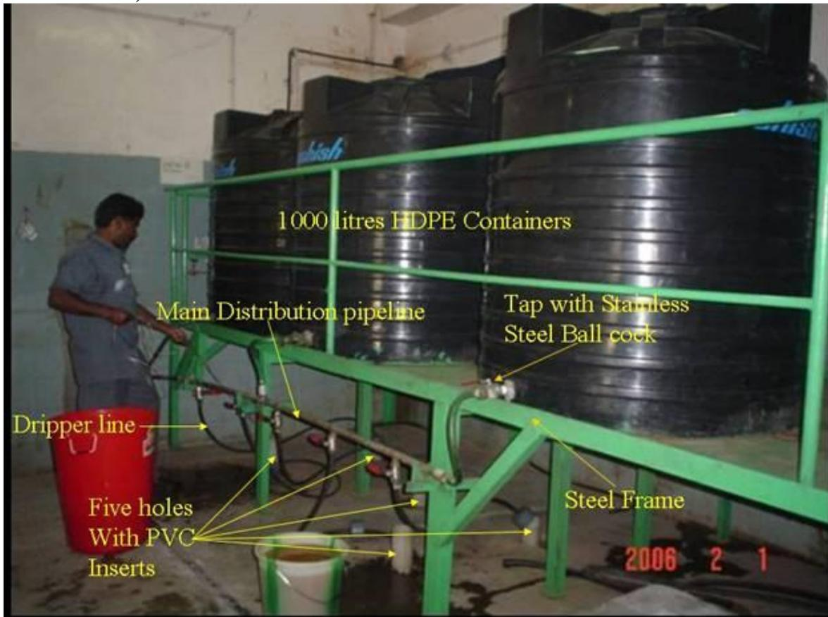
Fig 2. Structural set-up for carrying out dripping of SCD Bio Klean into holes
